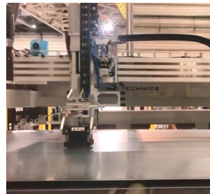
Control system for thickness, mechanical properties and laser marking
