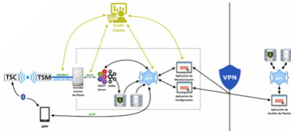
Solar structure control system scheme based on IoT elements
